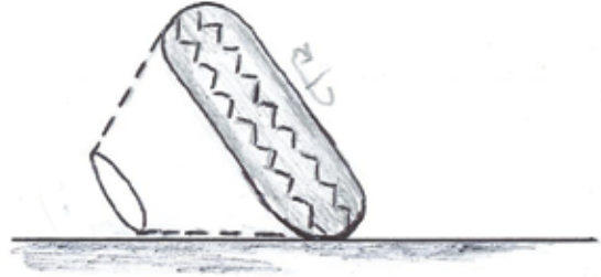
Figure 11: Because of its rounded cross-section, a rolling leaning tire behaves like a cone, helping the bike turn.
