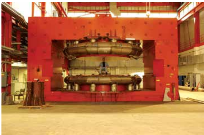
In this 2006 photo, Rutgers University graduate student Tim Koeth (now an assistant professor at the University of Maryland) sits between the poles of the Chicago Cyclotron Magnet at Fermi National Accelerator Laboratory. This type of magnet is typical of those used in high-energy physics experiments at the time of our SLAC experiment. Photo courtesy of Timothy Koeth.
