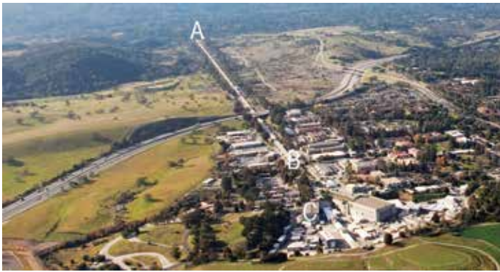
An aerial view of the SLAC facilities. The electrons started at (A) and traveled for 2 miles before reaching (B) with a beam energy of 16 GeV. The beam was then split and sent to different experiments; ours was housed at (C), known as End Station B. Photo by Brad Plummer, SLAC National Accelerator Laboratory.
