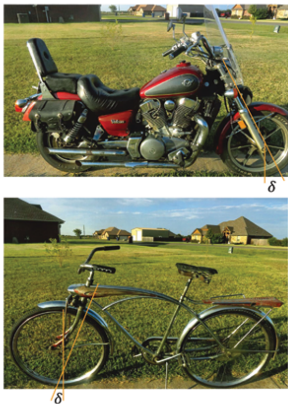
Figure 2 (from part I): Showing the castor distance on a 1994 Kawasaki Vulcan (top) and a 1962 J.C. Higgins Flightliner (bottom). Their front wheels have been deliberately set straight ahead. All photos and images by Dwight E. Neuenschwander unless otherwise noted.
