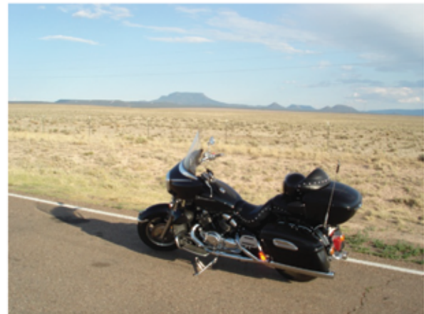
Figure 12: When leaning on the kickstand a bike's front wheel turns into the lean, as illustrated with a 2006 Yamaha Royal Star Midnight Venture near Pie Town, New Mexico.
