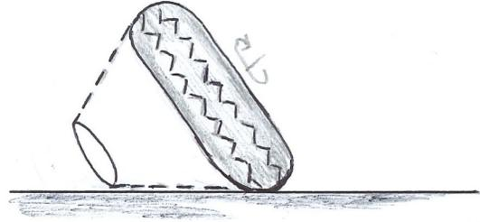
**Figure 11:** Because of its rounded cross-section, a rolling leaning tire behaves like a cone, helping the bike turn.
