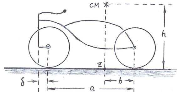
**Figure 4** (from part I): View of bike from the side, showing the distances  $a$ ,  $b$ ,  $h$ , and  $\delta$ .
