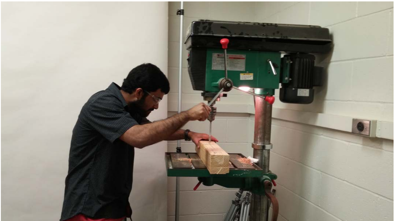
Figure 12: Kevin Cheriyan drilling holes into the plywood used as base in the slinky/ear demo.
