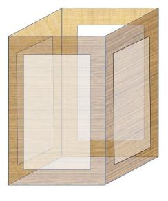
demonstrated the woodworking concept of maximizing sheet products and was made to be easily assembled and disassembled. Note that the structure, as shown, is structurally unsound. When built with full sheets of MDF, the sides will be fully rectangular, as shown in figure 2, to effect structural soundness.
