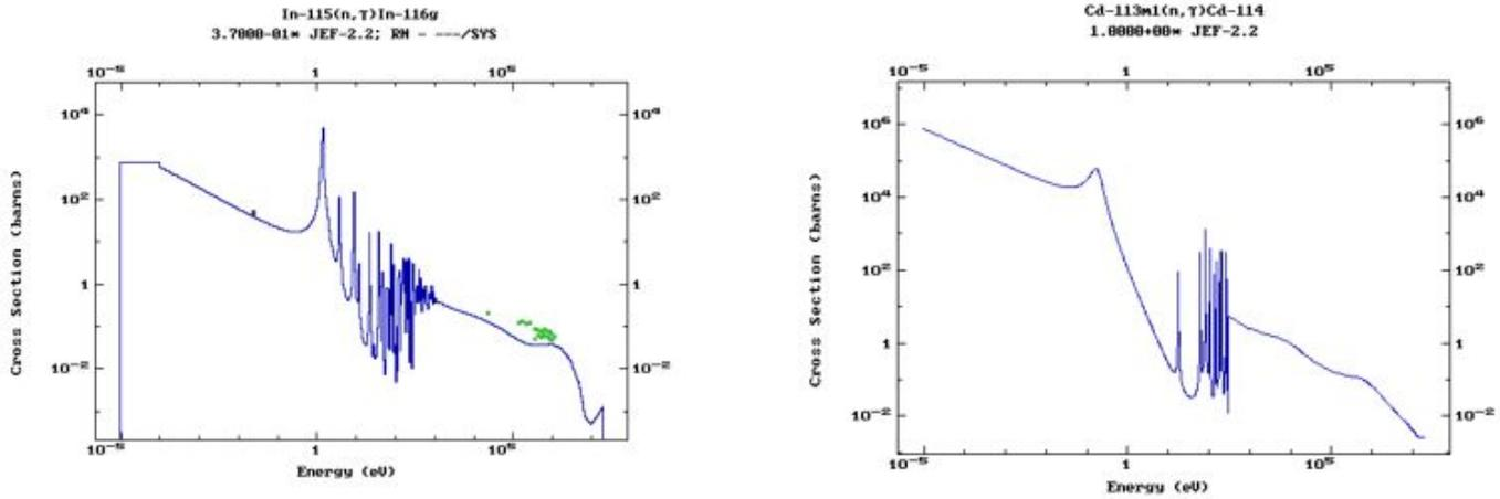
Figure 1 IAEA NGATLAS Atlas of Neutron Capture Cross Section (In-115 Left, Cd-113 Right)
