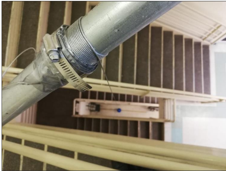
Figura 3. Provisional support of the prototype. The blue point at the center is the sphere.
